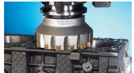
Roughing for cast iron
