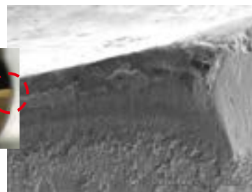
1000穴加工後の刃先 Flute tip after machining 1,000 holes
