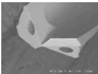
Tool wear after machining 1000 holes (25m)
