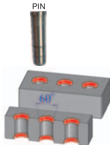
Chamfer with 60° used for deburring before "pin". 60° chamfer is easier than 90° or 120° to locate the pin.
