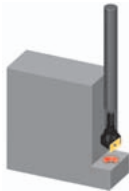
Chamfer cutter with longer shank
